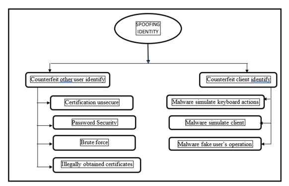
Figure 4. Threat analysis for external factors of spoofing with online banking client
